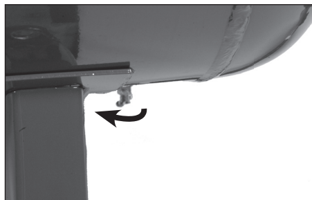
Figure 10 - Manual Tank Drain
